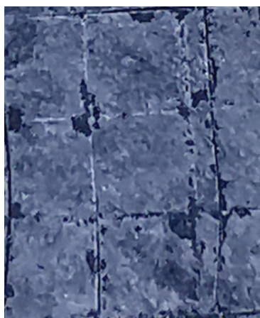
Fig. 5. Optical image of composite anHAp/TiO 2 coating after performing adhesion testing according to ASTM D 3359-02. 44
