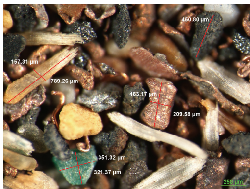
Fig. 2. Optical microscope pictures of the shaking table concentrate at \times 8 magnification.
