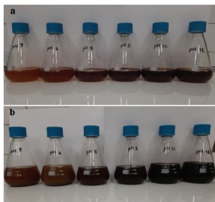
Fig. 4. a) The change in the color with changing pH of olive leaves extract in the pH range of 5.0–11.0 and b) silver nanoparticles synthesized using olive leaves extract in the pH range of 5.0–11.0 (60 min at 60 °C).
