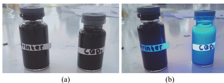
Fig. 6. Comparison under: a) normal light and b) 365 nm UV laser between N,B-codoped CQDs and commercial printer ink.
