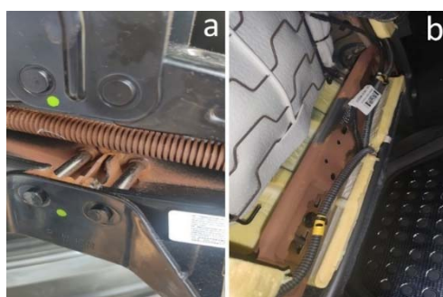
Fig. 2. Corrosion of: a) the automobile jack components and b) the frame and shaft inside.
