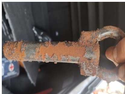
Fig. 6. Appearance of the applied organic coating (paint) on the surface of the towing hook.
