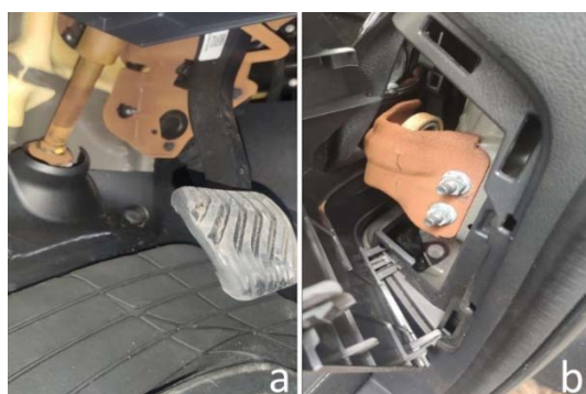
Fig. 3. Corrosion of: a) the steel components under the control panel and b) the steel parts under the protective mask on the rear seat.
