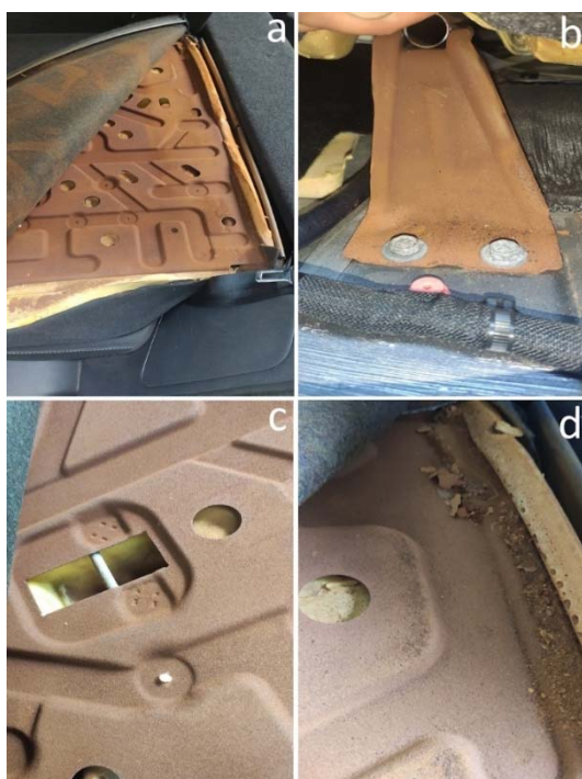
Fig. 4. Corrosion of steel parts.
