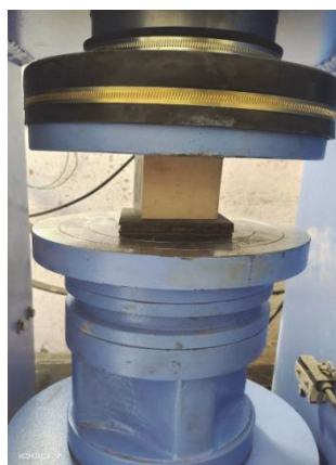
Fig. S-3. Compressive strength testing of MOC block by UTM machine.
