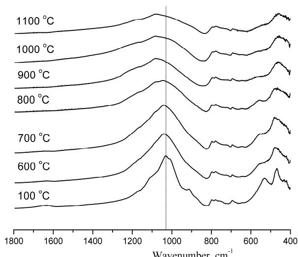
Fig. 3. FTIR spectra of raw clay from a locality near Pločnik excavation site, heated for 6 h at different temperatures; the vertical line marks the position of the Si–O stretching band at  $100\text{ }^{\circ}\text{C}$ .
