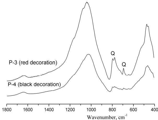
Fig. 5. Representative FTIR spectra (samples P-3 and P-4) of red and black decorations on pottery shards (Q – quartz).
