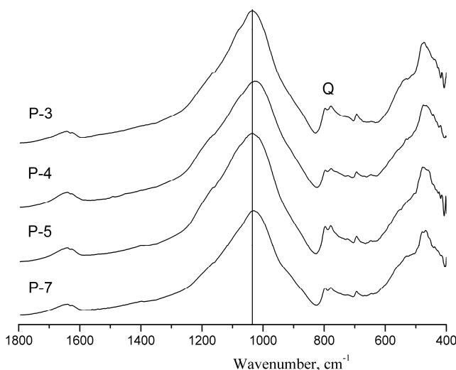
Fig. 2. FTIR spectra of representative pottery samples from Pločnik excavation site; Q designates quartz; the vertical line marks the position of the Si–O stretching band at 1040 cm<sup>-1</sup>.
