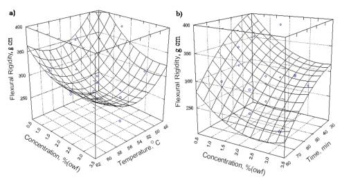
Fig. S-5. a) Effect of immobilized cellulase concentration and temperature on flexural rigidity, b) Effect of immobilized cellulase concentration and time on flexural rigidity.
