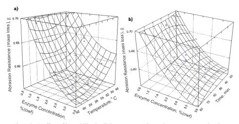
Fig. S-3. a) Effect of immobilized cellulase concentration and temperature on abrasion resistance b) Effect of immobilized cellulase concentration and time on abrasion resistance.
