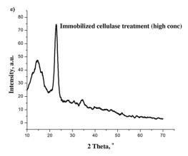
Fig. S-1. XRD spectra of a) Control fabric, b) Fabric treated with 1% concentration of free cellulase, c) Fabric treated with 3% concentration of free cellulase, d) Fabric treated with 1% concentration of immobilized cellulase, and e) Fabric treated with 3% concentration of immobilized cellulase.
