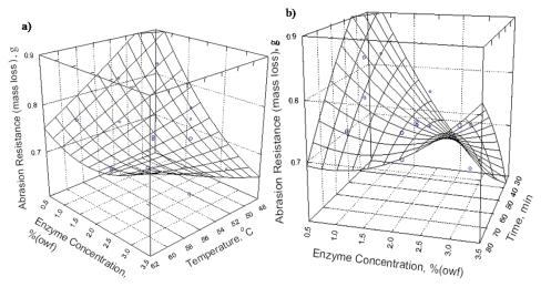
Fig. S-2. a) Effect of free cellulase concentration and temp on abrasion resistance b) Effect of free cellulase concentration and time on abrasion resistance.
