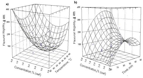
Fig. S-4. a) Effect of free cellulase concentration and temperature on flexural rigidity, b)
