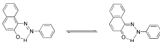
Fig. 2. Azo-hydrazone tautomerism of Sudan orange.
