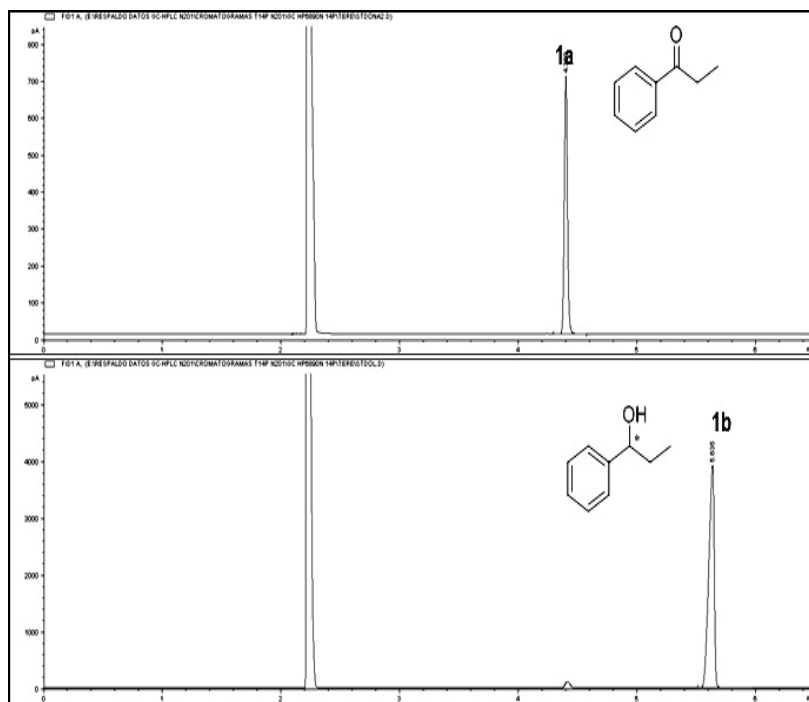
Fig. S-12. GC chromatograms of 1-phenyl-1-propanone ( 1a ) and 1-phenylpropan-1-ol ( 1b ).
