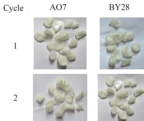
Fig. S-3. Images of the \text{PCL}_f+\text{TiO}_2 photocatalyst after repeated illumination cycles of dye (AO7 and BY28) solutions.
