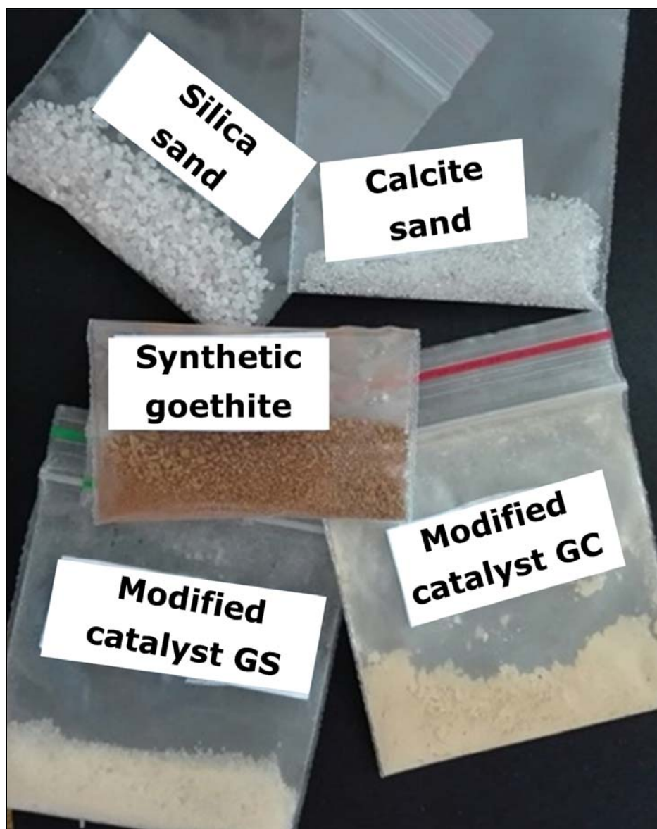
Fig. S-4. Photograph of synthetic goethite, the sands (silica and calcite) and the modified catalysts (GS and GC).
