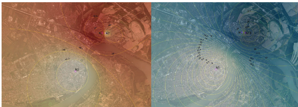
Fig. 6. The differences between measured and modelled fractions \phi of Chr and B(a)A for the city of Novi Sad, Serbia.
