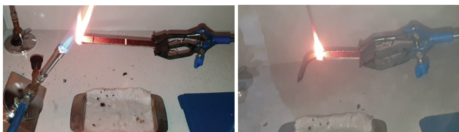
Fig. 7. PDA coated composite plate: A) ignition phase and B) propagation of the flame.
