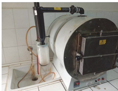
Fig. 2. PID controlled system producing BPL from biomass produced by mealworms.
