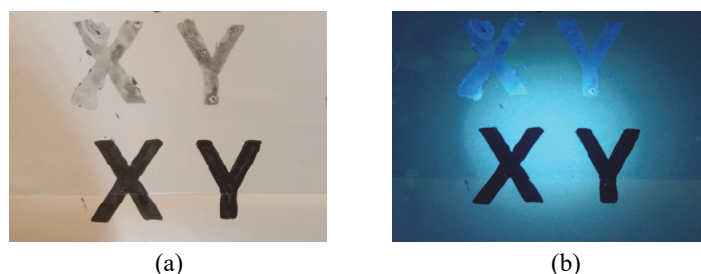
Fig. 7. Printed paper samples using N,B-codoped CQDs-based printer ink (top) and commercial printer ink (bottom) under: (a) normal lighting, and (b) UV 365 nm illumination.
