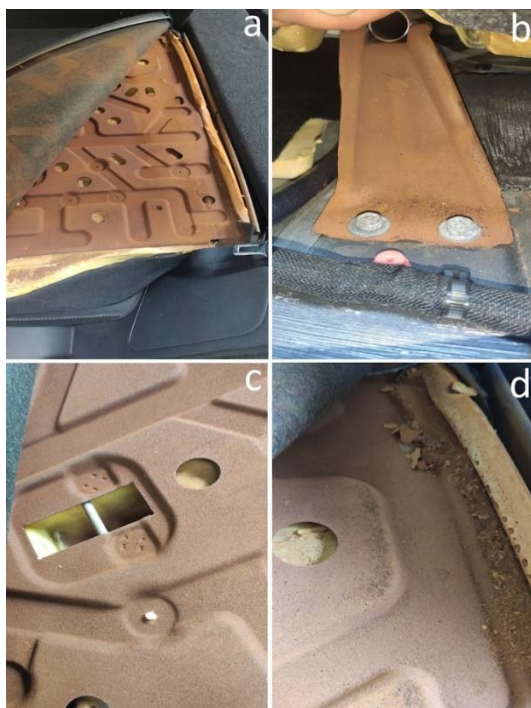
Fig. 4. Corrosion of steel parts.
